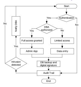
Fig: 2. MLC-DBS framework dataflow
